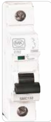
Knob : Mid Flag : Green Conclusion : Trip in case of fault
