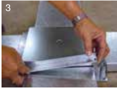
3 Align the trap frame bracket with the side blank plate
