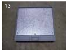
13 To convert the trap suitable for tile application, cut the tile according to the size of the trap.
